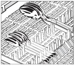
Spoon heads should be placed in contact with at least one of the serrated retainers on the base of the cutlery tray to ensure that water runs off them freely.
